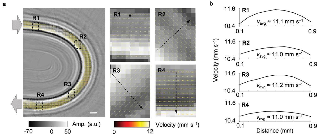
**Figure 7.** Ex vivo vector flow estimation by CRUST. a) Velocity map overlaid on the structural image of a U-shaped tube. R1 and R4 refer to the straight-tube regions near the entrance and exit. R2 and R3 represent the bent-tube regions. Magnified flow velocity vectors in R1–R4 are shown on the right. b) Velocity amplitude distributions along the line profiles in R1–R4. The computed average velocities are denoted by  $v_{\text{avg}}$ . Scale bars = 1 mm; Amp. = amplitude.
